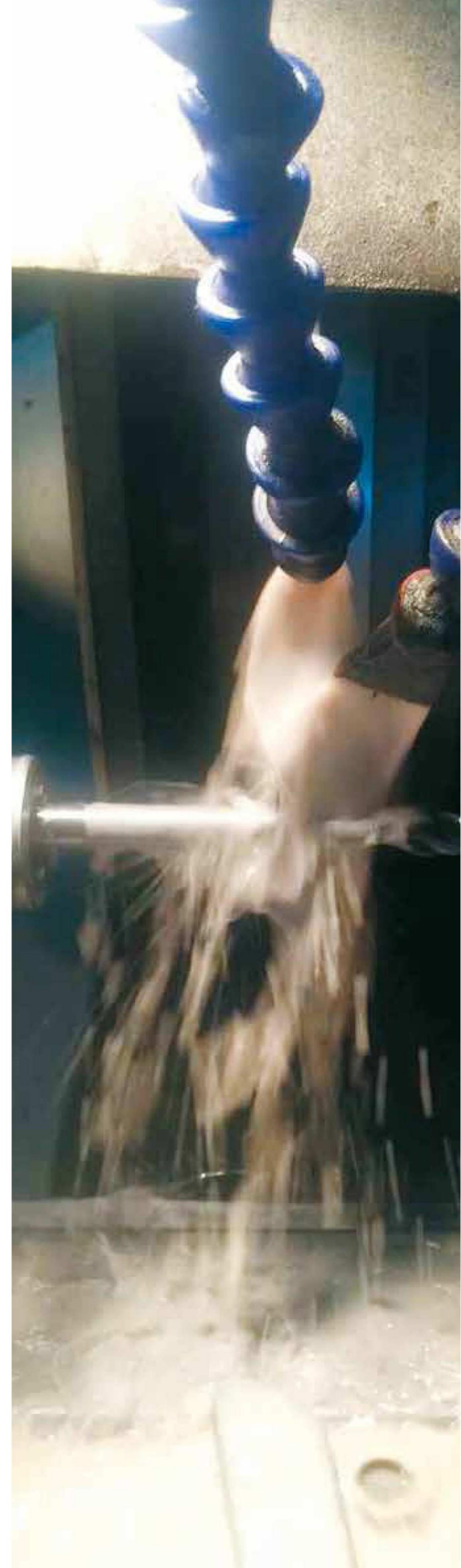
Different tool holder interfaces can be selected according to the customer's different machine tool rigidities, such as heat-shrinkable, integrated, flange adapter, etc. The tool is factory-set with a dynamic balance level of G2.5 and is equipped with internal cooling holes to increase the service life of the tool.
